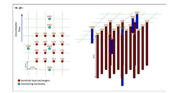
The storage is located in the area of an open operational hall next to the previously existing gas boiler room and consists of 21 boreholes, the 16 of which are BHEs (charging/discharging, V01 – V16) and 5 of which are monitoring (VM1 – VM5)
