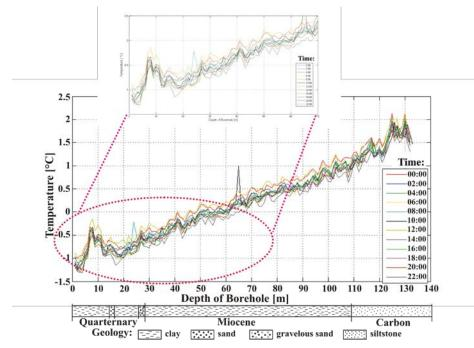
Data record of the temperature changes after the optical cable installation for measurement of the temperature changes in the rock massif with respect to the depth and phase (during heat offtake).
